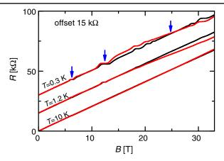
FIG. 3. Comparison of  $R_{xy}$  (black) and the inverted resistance rule  $R_{diff}^{-1}$  (red) for 0.3 K, 1.2 K and 10 K. For clarity the curves have been offset with respect to each other. The blue arrows indicate from left to right the positions of the filling factors  $\nu = 2$ , 1 and 1/2, respectively.
